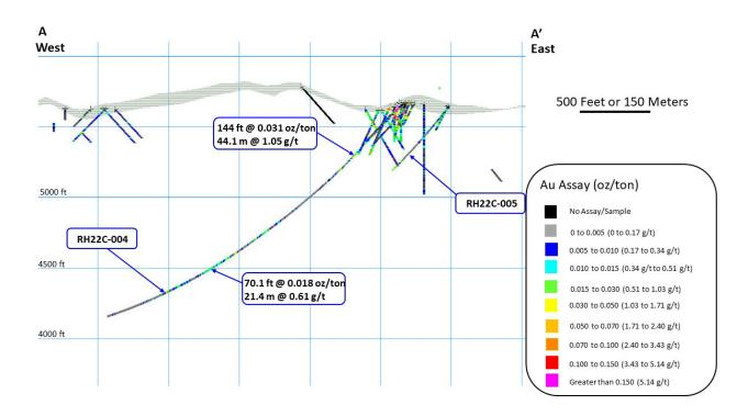
Figure 5. Cross Section View of RH22C-005 and historical drilling along B-B in Figure 3.
